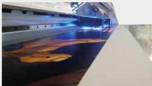
Lampade UV Led un asciugatura istantanea UV Led lamps for instantaneous drying
